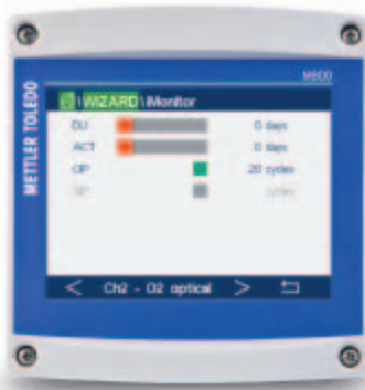
Fig. 3: iMonitor display on M800 transmitter
