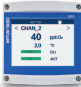
Fig. 2: M800 display showing DLI and ACT sensor diagnostics
