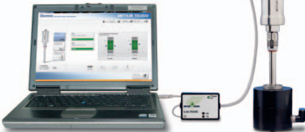
iSense software calibrating a dissolved oxygen sensor
